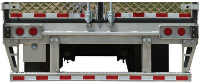
The new rear underride guard comes standard with no additional cost and weight. It resists compartmental intrusion of an automobile when the location of impact is at 30% to 100% overlap of the width of the car to the guard. It complies with all applicable U.S. and Canadian regulations. The bolt-on design allows for easy repairability.
